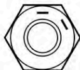
Two circumferential lines located 60° apart
